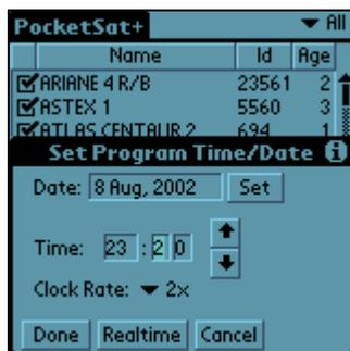
The PocketSat+ clock is the heart of the application, and drives everything else. Visible at the lower right corner of the screen in all program modes, it can be set by tapping either the date or time display.
