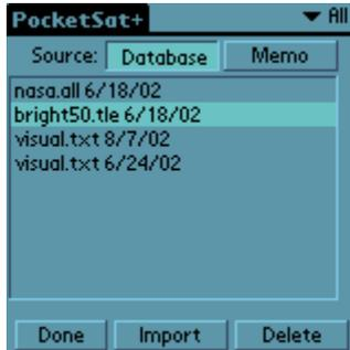
PocketSat keeps an internal database containing satellite orbital data. As the data ages, it is periodically necessary to replace it with new data. This is done by pressing the “Import” button on the main Satellites form. If an imported dataset includes a satellite that is already in the PocketSat+ database, the old data will simply be overwritten, so there is no need to delete old data before performing an import.
