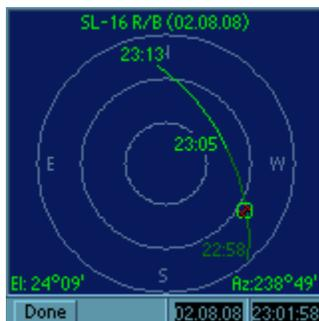
Pressing the “Plot” button brings up a plot of the sky which shows the satellite's path across the sky during the pass. This plot is in most ways identical to the Sky mode, the only real difference being that rise, set and culminations times for the pass are displayed on the plot.
